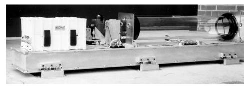
Figure 3. *The spectrometer before it was placed into the airplane.*
