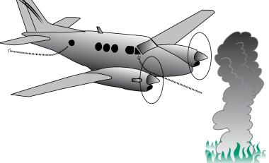
Figure 4. Example of the duct system showing how forest fire smoke was moved through the spectrometer as the airplane flew through forest fire smoke.
