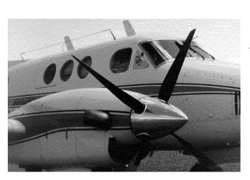
Figure 2. USDA Forest Service Air King 90. The smoke intake is visible in the side cockpit window. The pilot sat on the other side of the cockpit.
