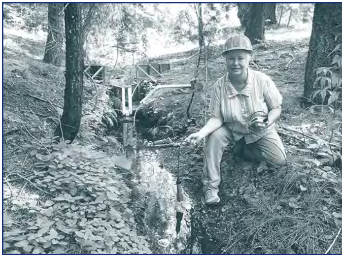
Figure 11. Dr. Hunsaker holds an instrument that measures water acidity, water temperature, and the amount of dissolved substances in a stream within the Kings River Experimental Watersheds. A flume sits in the stream behind her. The flume creates a uniform streamflow so that scientists can measure the amount of water flowing in the stream. Solar-powered instruments automatically measure and record the amount of streamflow every 15 minutes. Photo courtesy of Dr. Carolyn Hunsaker.
