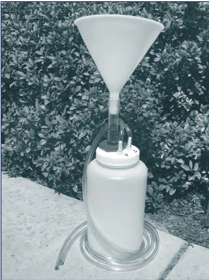
Figure 14. This snowmelt sampler is used to collect snowmelt. These samplers are buried in the soil up to the base of the funnel. An air line and a sample line are connected to the funnel. When it snows and the snow melts, the water sample is pumped out by hand. Photo courtesy of Dr. Carolyn Hunsaker.
