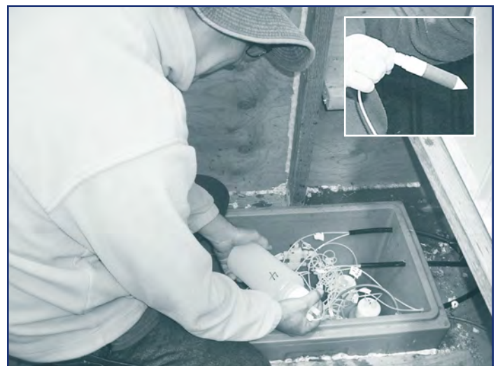
Figure 13. This scientist is preparing vacuum pumps that enable him to collect soil water. The tip shown in the inset is inserted into the soil to collect the water. Photo courtesy of Dr. Carolyn Hunsaker.
