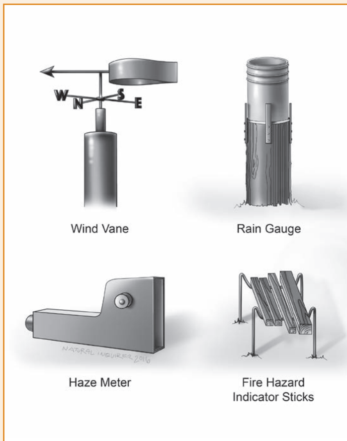
Figure 21. Fire guards used wind vanes, haze meters, rain gauges, and hazard indicator sticks as tools to measure the danger of wildland fire. Wind vanes measure wind speed and direction. Haze meters measure the distance at which smoke from a wildland fire can be seen from a location. Rain gauges measure the amount of rainfall in a location. Fire hazard indicator sticks help measure the dryness of different types of wood.
