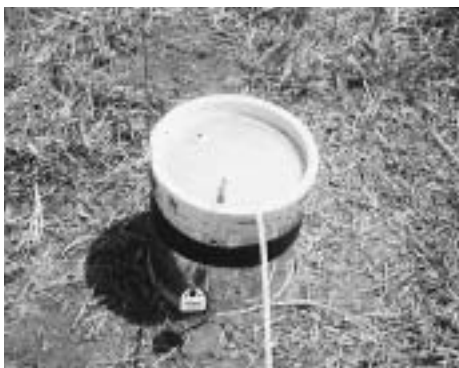
Figure 6. Photograph of equipment used to collect nitrous oxide gas.
