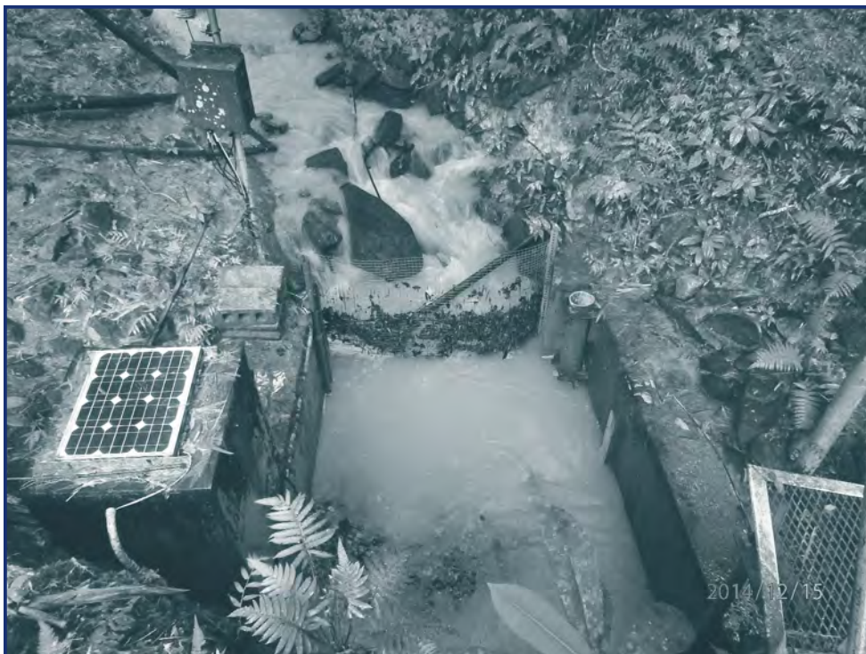
Figure 13. Mesh traps were placed across the stream channels to collect coarse particulate organic matter (CPOM). Photo courtesy of Tamara Heartsill Scalley.
