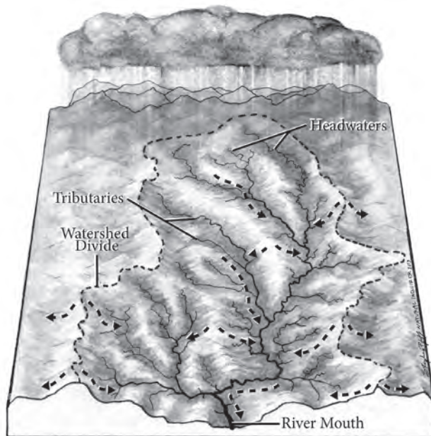
FIGURE 1. A WATERSHED IS AN AREA OF LAND WHERE ALL OF THE WATER THAT IS UNDERGROUND WITHIN THE AREA, AND ALL OF THE WATER IN STREAMS AND RIVERS IN THE AREA, FLOWS TO THE SAME PLACE. ILLUSTRATION BY STEPHANIE PFEIFFER.
