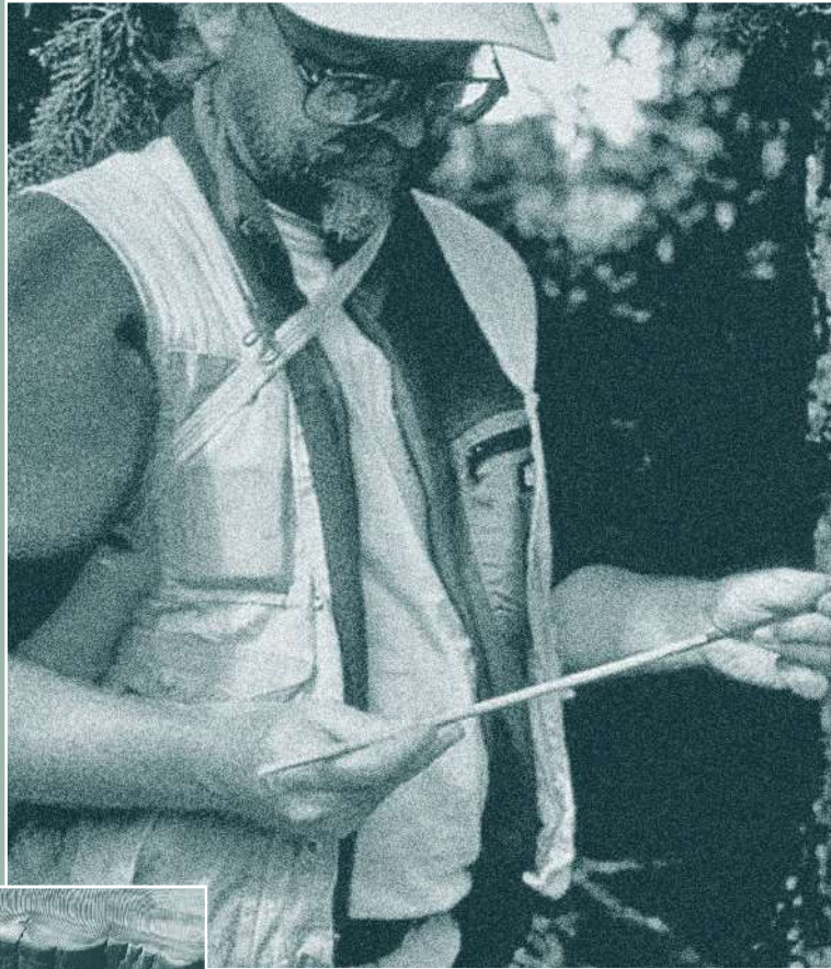
Figure 4. Dendrochronologists do not have to kill trees to get information from tree rings. An increment borer allows scientists to pull a small sample of the tree’s rings. The hole created by the borer is then sealed to protect the tree. The sample is a long, thin cylinder of wood. Photo courtesy of Edward Cook and the National Oceanic and Atmospheric Administration (NOAA) Paleoclimatology Program, U.S. Department of Commerce.
