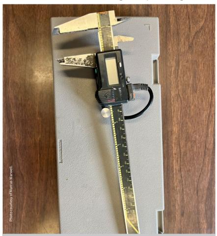
These are calipers. The tips of the calipers open to measure how big a plant is. These calipers can send the measurements to a computer that Dr. Warwell used.
