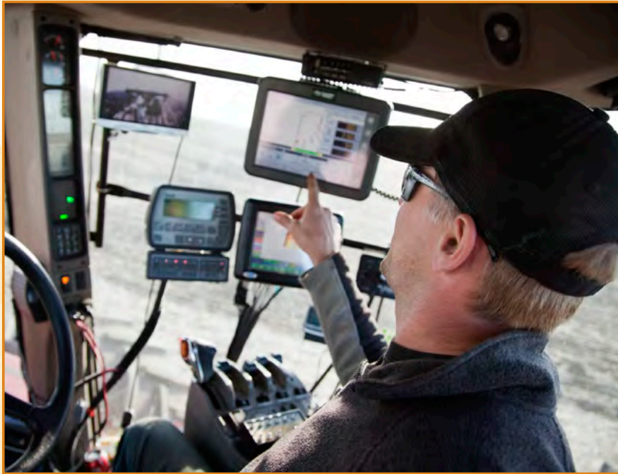
Figure 14. A Case IH AFS PRO-600 is a computer mounted to the machinery which farmers use to harvest crops. The computer calculates the quantity of crops being harvested, among other things.
