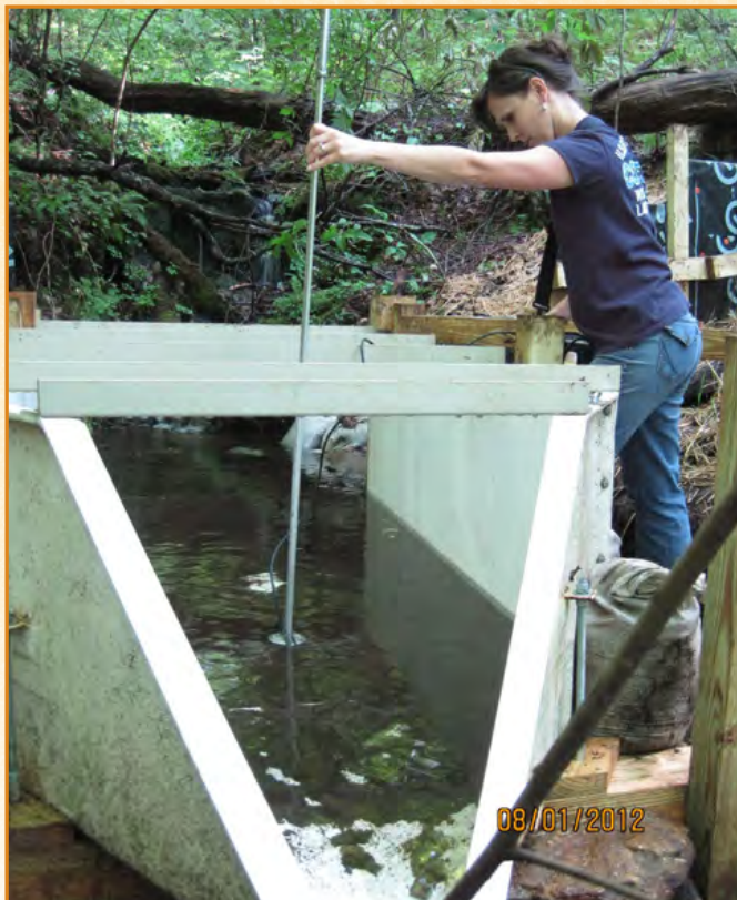
Figure 13a. An H flume is placed in a stream to calculate water flow. The H flume forces all water into one space so scientists can accurately measure how much water is flowing in a particular location.
