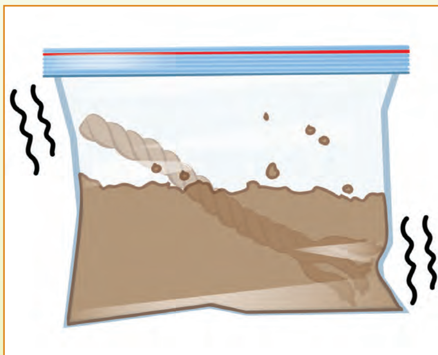
Figure 20. Place each piece of rope individually into the bag and shake for 10 seconds. Remove the rope and place it on the table until each rope has been shaken and compared to one another.
